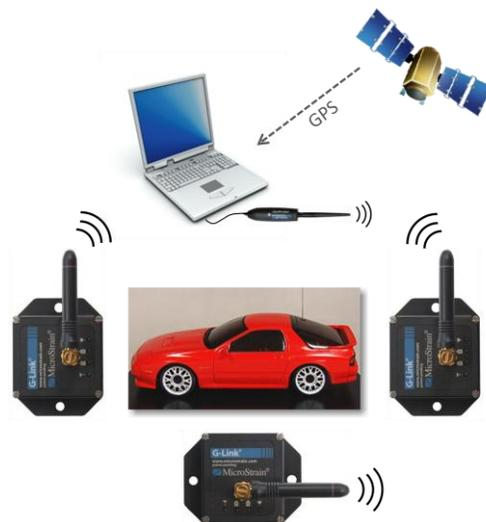
Figure 1: Schematic of organization of sensors and coordination computer.
