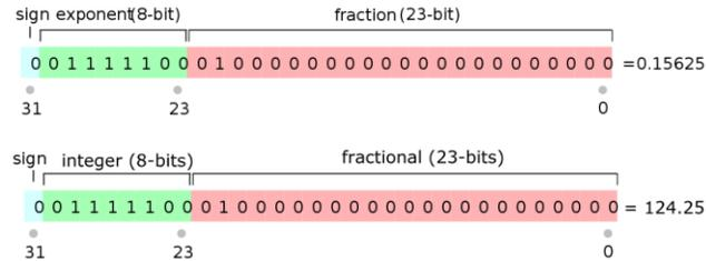
Figure 7: Layout of IEEE 754 floating-point representation and arbitrary fixed point representation.
