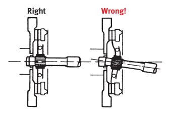
Worn splines on the transmission input shaft will cause erratic movement during load changes, which can bend tangential leaf springs and cause disengagement problems or juddering.
