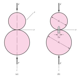
These equations are valid for either sphere, but the value used for Poisson's ratio must correspond with the sphere under consideration. The equations are even more complicated when stress states off the z axis are to be determined, because here the x and y coordinates must also be included. But these are not required for design purposes, because the maxima occur on the z axis.
