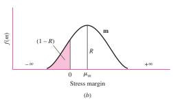
1 - R where parts are expected to fail. We next consider some typical cases involving stress-strength interference.
