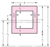
$$r_c = r_i + \frac{\frac{1}{2}h^2t + \frac{1}{2}t_i^2(b-t) + t_o(b-t)(h-t_o/2)}{ht + (b-t)(t_i + t_o)}$$
