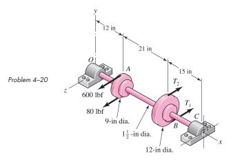
**4–21** The figure shows a steel countershaft that supports two pulleys. Pulley C receives power from a motor producing the belt tensions shown. Pulley A transmits this power to another machine through the belt tensions  $T_1$  and  $T_2$  such that  $T_1 = 8T_2$ .
