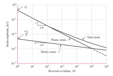
The report contains a plot of this relationship for SAE 1020 hot-rolled steel; the graph has been reproduced as Fig. 6–13. To explain the graph, we first define the following terms:
