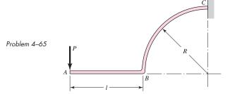
**4–66** For the wire form shown determine the vertical deflections of points *A* and *B*. Consider bending only and assume Eq. (4–28) applies.
