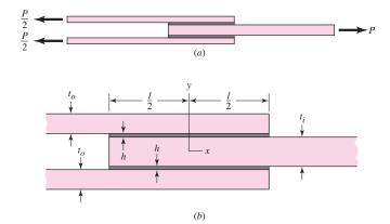
illustrate the principles. The shear-stress distribution for the double lap joint of Fig. 9–26 is given by
