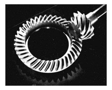
It is frequently desirable, as in the case of automotive differential applications, to have gearing similar to bevel gears but with the shafts offset. Such gears are called *hypoid gears*, because their pitch surfaces are hyperboloids of revolution. The tooth action between such gears is a combination of rolling and sliding along a straight line and has much in common with that of worm gears. Figure 15–3 shows a pair of hypoid gears in mesh.
