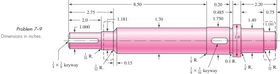
7-10 An AISI 1020 cold-drawn steel shaft with the geometry shown in the figure carries a transverse load of 7 kN and a torque of 107 N · m. Examine the shaft for strength and deflection. If the largest allowable slope at the bearings is 0.001 rad and at the gear mesh is 0.0005 rad, what
