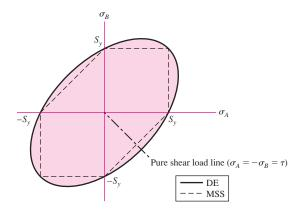
Equation (5–13) is a rotated ellipse in the  $\sigma_A$ ,  $\sigma_B$  plane, as shown in Fig. 5–9 with  $\sigma' = S_y$ . The dotted lines in the figure represent the MSS theory, which can be seen to be more restrictive, hence, more conservative.<sup>4</sup>
