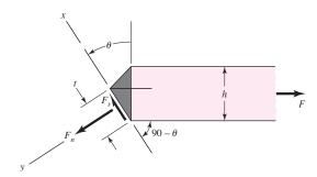
The average stress in a butt weld due to shear loading (Fig. 9–7b) is
