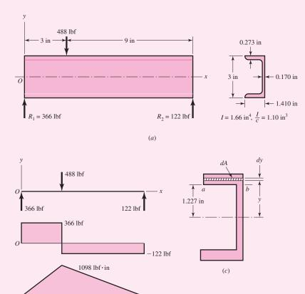
Solution The loading, shear-force, and bending-moment diagrams are shown in Fig. 3–19b. If the direct shear force is included in the analysis, the maximum stresses at the top and bottom of the beam will be the same as if only bending were considered. The maximum bending stresses are
