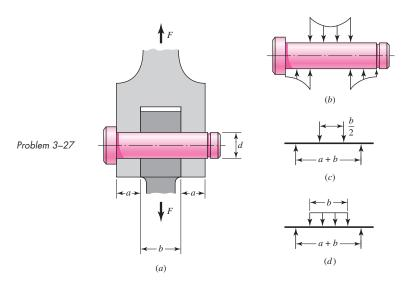
**3–28** The figure illustrates a pin tightly fitted into a hole of a substantial member. A usual analysis is one that assumes concentrated reactions R and M at distance l from F. Suppose the reaction is distributed linearly along distance a. Is the resulting moment reaction larger or smaller than the concentrated reaction? What is the loading intensity q? What do you think of using the usual assumption?
