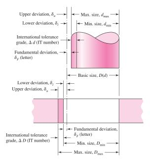
• *Shaft basis* represents a system of fits corresponding to a basic shaft size. The fundamental deviation is h. The shaft-basis system is not included here.
