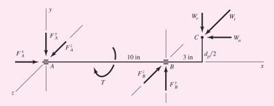
These three forces,  $W_r$  in the -y direction,  $W_a$  in the -x direction, and  $W_t$  in the +z direction, are shown acting at point C in Fig. 13–39. We assume bearing reactions at A and B as shown. Then  $F_A^x = W_a = 23.3$  lbf. Taking moments about the z axis,
