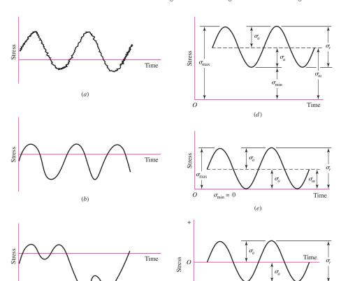
Figure 6–23 illustrates some of the various stress-time traces that occur. The components of stress, some of which are shown in Fig. 6–23*d*, are
