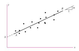
where m is the slope and b is the y intercept. Consider a set of N data points  $(x_i, y_i)$ . In general, the best-fit line will not intersect a data point. Thus, we can write
