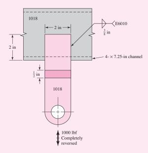
In the absence of a midrange component, the fatigue factor of safety  $n_f$  is given by
