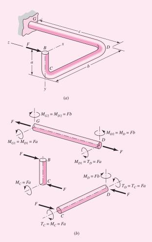
appropriate use of *free-body diagrams* is essential here. The reader should verify that the reactions as functions of F in elements BC, CD, and GD are as shown in Fig. 4–11b. The deflection of B in the direction of F is given by
