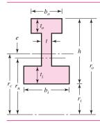
$$r_c = r_i + \frac{\frac{1}{2}h^2t + \frac{1}{2}t_i^2(b_i - t) + t_o(b_o - t)(h - t_o/2)}{t_i(b_i - t) + t_o(b_o - t) + ht}$$
