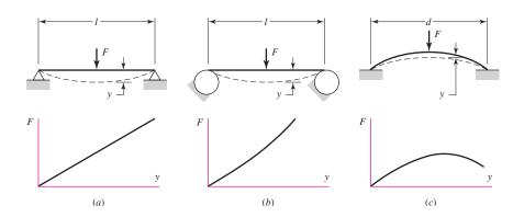
Figure 4–1c is an edge-view of a dish-shaped round disk. The force necessary to flatten the disk increases at first and then decreases as the disk approaches a flat configuration, as shown by the graph. Any mechanical element having such a characteristic is called a *nonlinear softening spring*.
