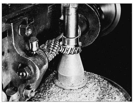
and cutter roll slightly on their pitch circles. When the blank and cutter have rolled a distance equal to the circular pitch, the cutter is returned to the starting point, and the process is continued until all the teeth have been cut.
