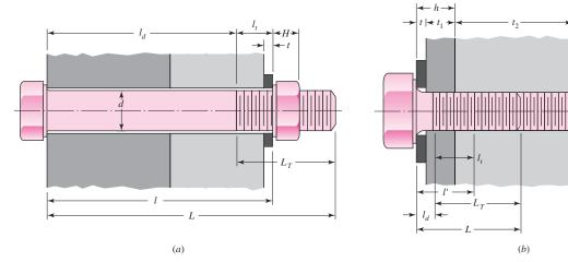
Given fastener diameter d and pitch p or number of threads
