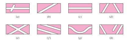
oil in at the center of the bushing so that it will flow out both ends, thus increasing the flow and cooling action.
