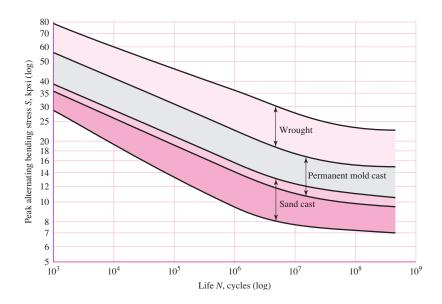
The ordinate of the S-N diagram is called the *fatigue strength*  $S_f$ ; a statement of this strength value must always be accompanied by a statement of the number of cycles N to which it corresponds.
