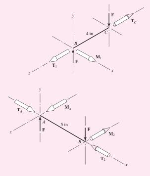
(b) For arm BC, the bending moment will reach a maximum near the shaft at B. If we assume this is 1200 lbf  $\cdot$  in, then the bending stress for a rectangular section will be
