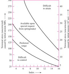
$L_0$  and  $F_i$  is the initial tension in the spring that must be exceeded before the spring deflects. The load-deflection relation is then
