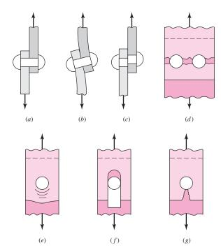
this manner is an assumption, because we do not know exactly how the load is distributed to the rivet or the relative deformations of the rivet and the members. Although this equation can be used to determine the bending stress, it is seldom used in design; instead its effect is compensated for by an increase in the factor of safety. In Fig. 8–23c failure of the rivet by pure shear is shown; the stress in the rivet is
