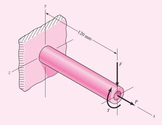
Solution Since the maximum bending moment is M = 120F, the normal stress, for an element on the top surface of the tube at the origin, is
