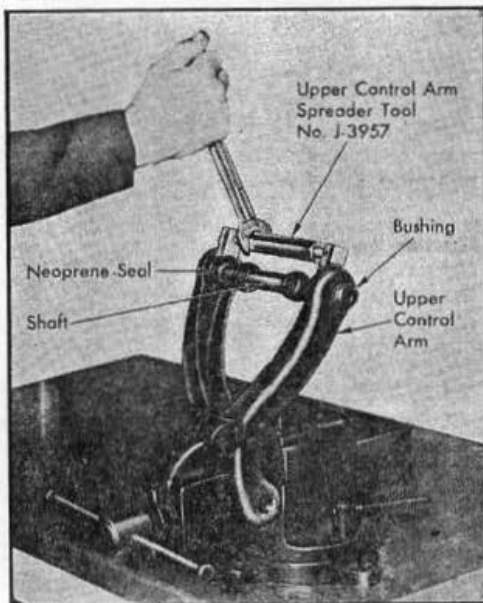
Fig. 38 Spreading upper control arm, 1950-54
